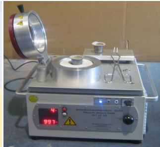
D 80 : Equipment to measure the density solidified at 80 mbar.
