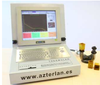
Thermolan-AI : Equipment to measure the modification of eutectic Si.
