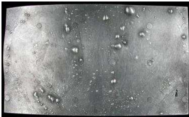
Blistered 2 mm plate made of EN-AC-AISI9Cu3
