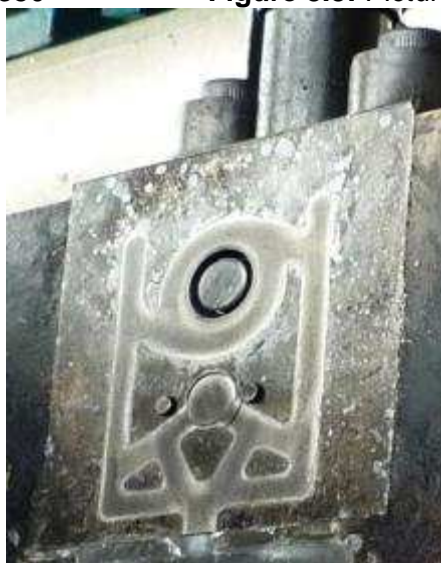
Figure 3.5: Vacuum valve with control piston and ejector pins - cover die half
