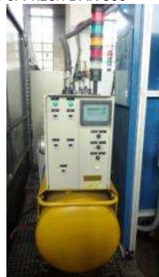
Figure 3.6: Vacuum tank with control unit and vacuum pump
