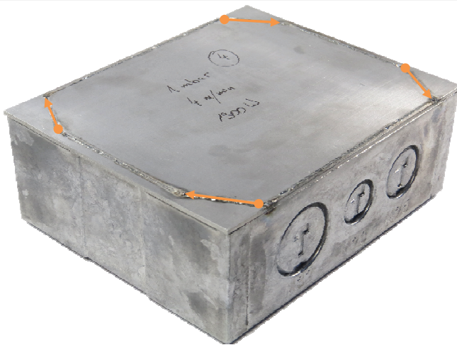
Figure 3.8: Weld bead position for tack welding
