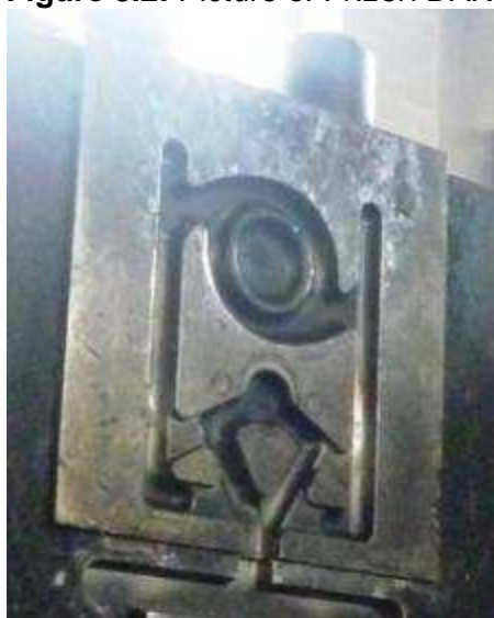
Figure 3.4: Typhoon vacuum runners - ejector die half
