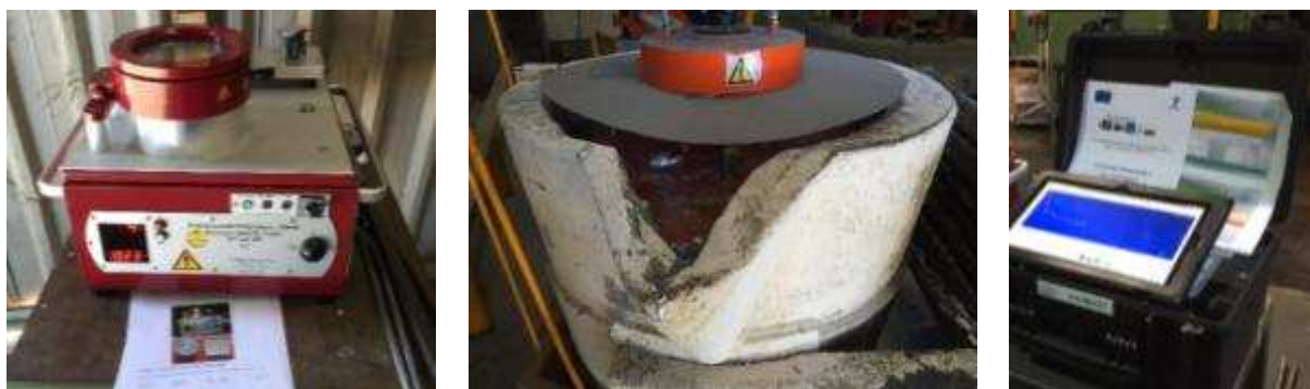
Figure 2.5 Images of the vacuum tester used for controlling the metal quality (left), the rotor used for the degassing treatment (centre) and the thermal analysis equipment (right).
