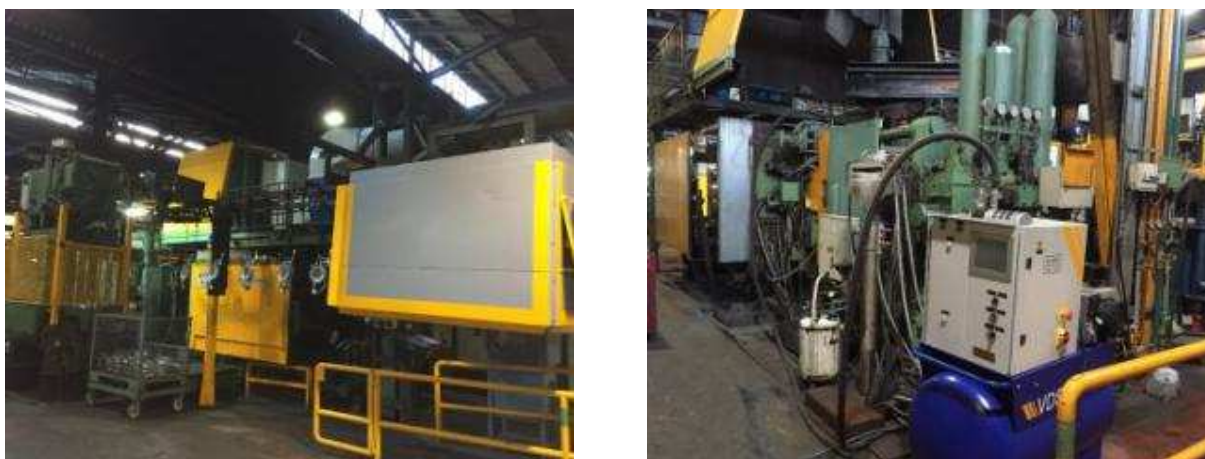
Figure 2.7 Image of the die casting machine, 700 tn (left), and the vacuum equipment, VDS PLC 350 (right), used to cast Ruffini's demonstrator.
