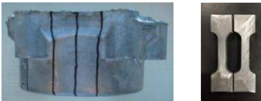
Figure 2.13. Tensile test samples obtained from each Ruffini's demonstrator.
