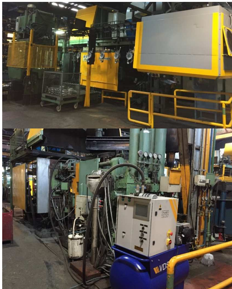
Figure 5.2 Die casting machine, 700tn and Vacuum unit VDS PLC 350.
