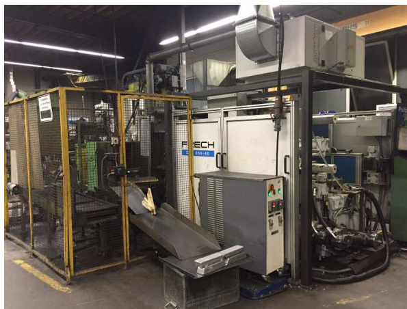
Figure 3.2 HDPC production unit of Schmale & Schulte
