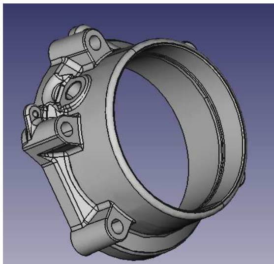
Figure 2.1 3D CAD image of the component selected by RUFFINI for the demonstration activity of Soundcast project (High mechanical properties demonstrator).
