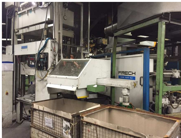
Figure 3.4 HDPC production unit with of Schmale & Schulte
