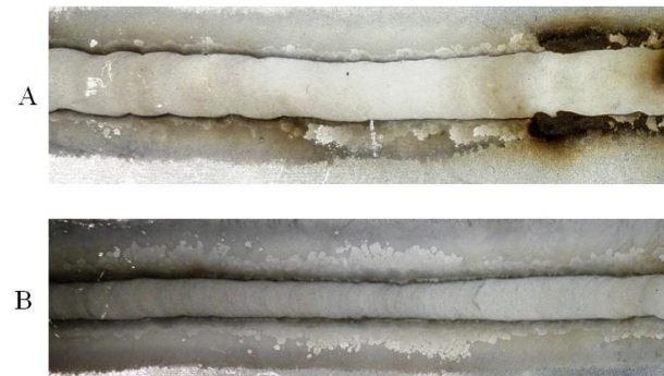
Fig. 12. Details of the re-melt seam in the area opposite the ingate A) conventional; B) minimal die lubrication
